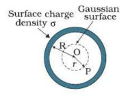
In this case, the Gaussian surface encloses no charge. Gauss's law then gives  $E \cdot 4 \pi r^2 = 0$ i.e., E = 0, (r < R)
