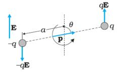
Consider a permanent dipole of dipole moment p in a uniform external field E. There is a force qE on q and a force -qE on -q.
